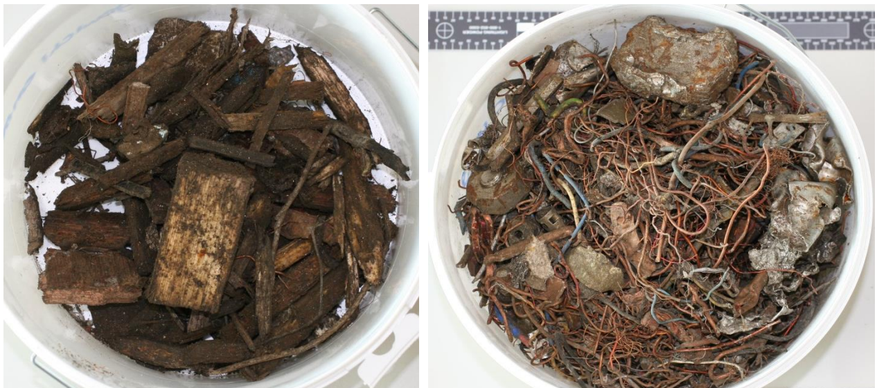
Photo 4 Visible contamination of aluminium scrap. The material was unduly being exported from the Netherlands to China as Green listed (not mixed material) under the Waste Shipment Regulation (WSR) (photo NFI)
