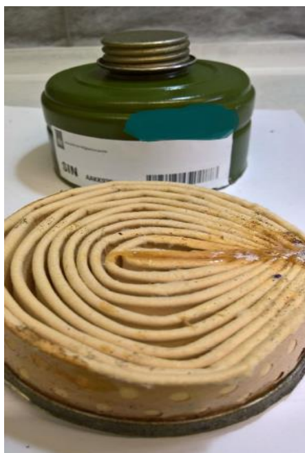
Photo 5 Import into the Netherlands from Eastern Europe of old army filter canisters. Besides the common asbestos type chrysotile the filters also contain the rarer richterite and winchite fibres (picture SEM (Scanning Electron Microscope) on the right). The latter are asbestos like fibres but not regulated (Photos: NFI)
