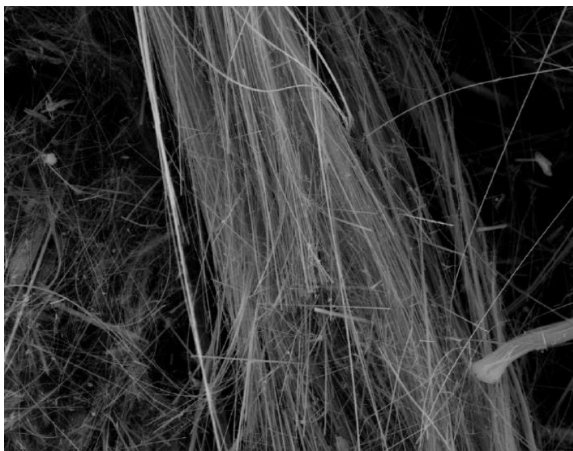
Photo 5 Import into the Netherlands from Eastern Europe of old army filter canisters. Besides the common asbestos type chrysotile the filters also contain the rarer richterite and winchite fibres (picture SEM (Scanning Electron Microscope) on the right). The latter are asbestos like fibres but not regulated (Photos: NFI)
