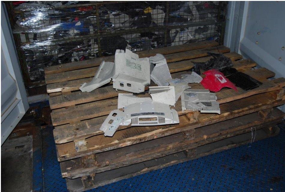
Photo 2 Illegal export of hazardous WEEE with brominated flame retardants (photo NFI). Detection has taken place with a mobile XRF (X-ray fluorescence)
