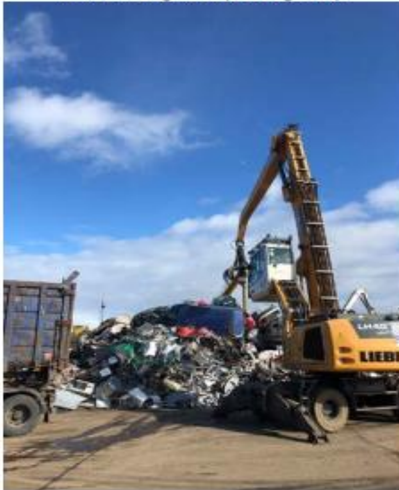
Mechanical grab separating scrap
