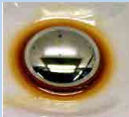
Photo 27: Elemental mercury in methamphetamine waste. Photo: NFI
