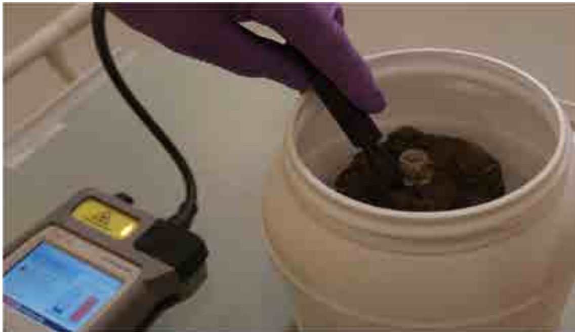
Photo 3: Use of the laser pointer of a mobile Raman. Photo: NFI.
