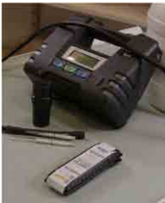
Photo 4: Dräger-Tubes in combination with an electrical pump. Photo: NFI.
