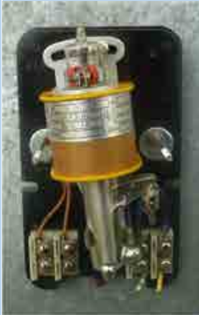
Photo 37: Closed mercury relay, with a coil around the top of the tube and adjustable angle. Photo: internet A. Dingley
