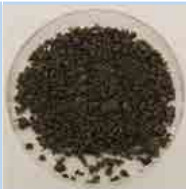
Photo 23: Dental amalgam spilling from dental treatment. Material obtained from BMT International (The Netherlands). BMT is specialized in developing practical Total Mercury management solutions for mercury containing wastes. Photo: NFI.
