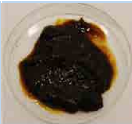
Photo 22: Mercury butter from mercury cell chlor-alkali production. Material is obtained from BMT International (The Netherlands). BMT is specialized in developing practical Total Mercury management solutions for mercury containing wastes. Photo: NFI.
