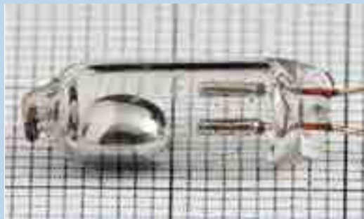
Photo 33: Mercury switch. Mercury switches have one or more sets of electrical contacts in a sealed glass envelope that contains elemental mercury. Photo: Mercury switch - Wikipedia .
