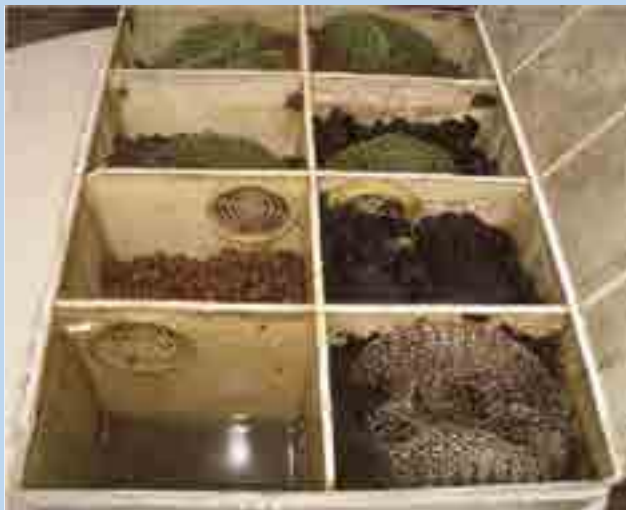
Photo 25: Amalgam separator interior. Designs are variable. Source: (Hylander L. , Lindvall, Uhrberg, Lindh, & Gahnberg, August 2006).
