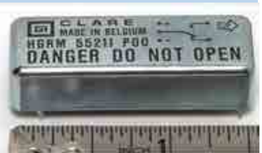
Photo 34: Mercury wetted relay. Other models can be found in (Naturvardsverket, november 2003). Photo: File:Clare HGRM-55211-P00 mercury-wetted reed relay.jpg - Wikimedia Commons
